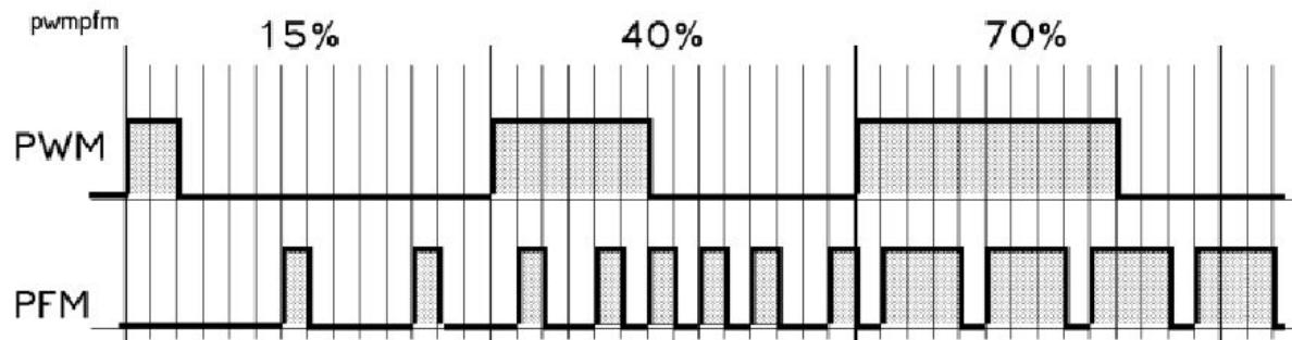
For getting very low motor speed, PFM pulses must be long enough to bring enough energy to make the motor win against frictions. Hence, there is no limit to minimal speed, but movement is cogged. For speed of few %, the gearbox will smoothe it.
