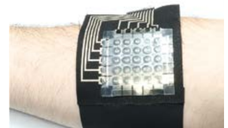
Haxel array with textile printed circuit board sleeve.
