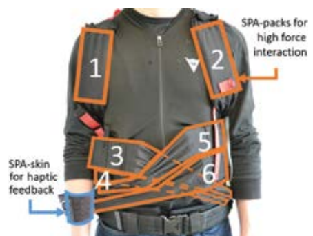
A completely soft robotic exosuit with two kinds of soft pneumatic actuation for a high fidelity tactile feedback (blue) and posture support with up to 100 N force output per unit (orange).
