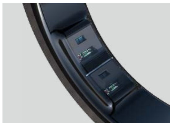
Incorporation of the world's smallest PPG chips, enabling eighteen light sources and six sensors to be integrated around the perimeter of the ring.
