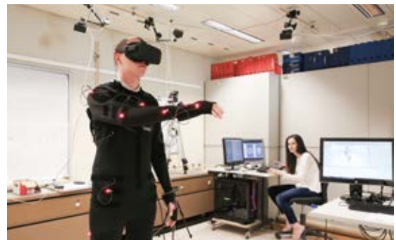
This experimental system is used to quantify human sensitivity to distortions in our posture when displayed in the VR headset.
