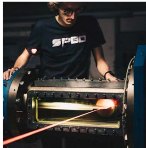
Hydrofoil tests in the LMH cavitation tunnel – © Guillaume Fischer.
