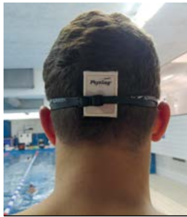
Body-fixed inertial measurement unit for the head.
