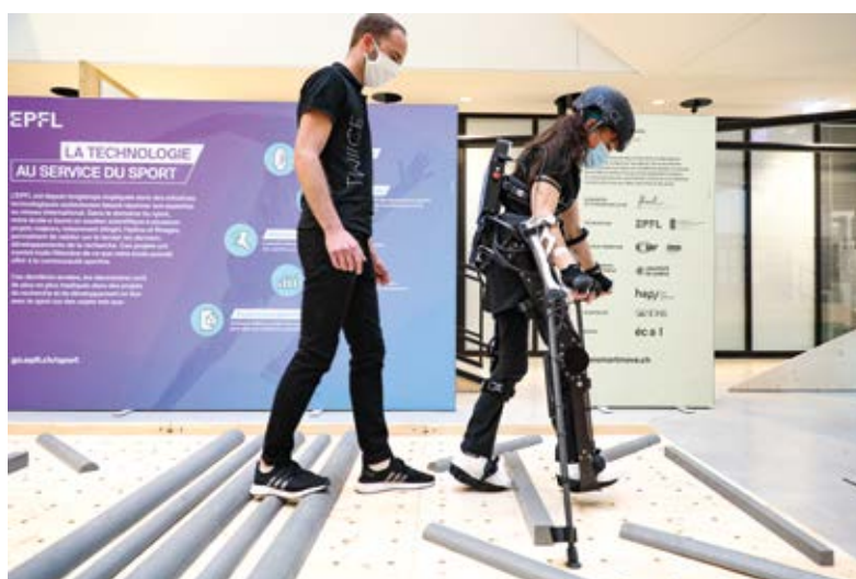
The Twice One exoskeleton allows people with paraplegia – complete paralysis of the lower limbs – to stand up and walk using motors on each leg.
