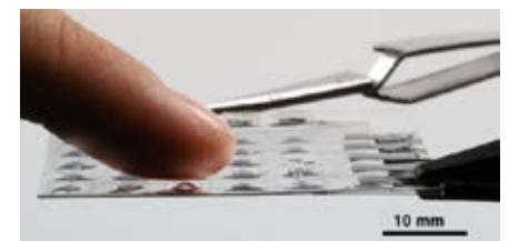
Hydraulically amplified zipping electrostatic actuators, or Haxels capsules.
