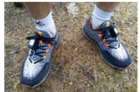
Foot-worn inertial measurement units (Physilog 5).
