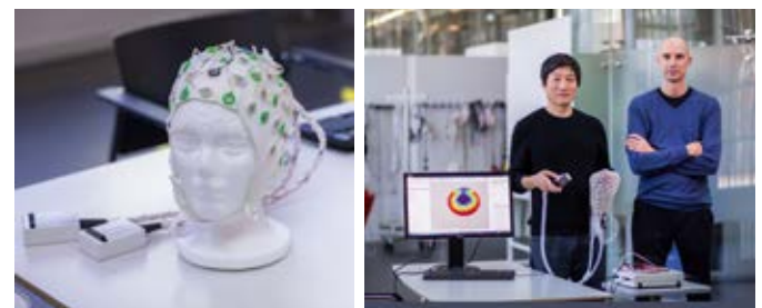
Headset for measuring brain activity and signal of readiness potential (RP).
