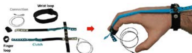
Thin high-force textile electrostatic clutches.
