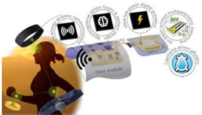
WeCare, wearable sweat sensing platform.
