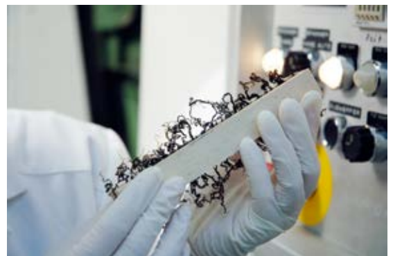
Sample of welded wood.
