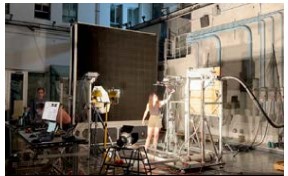
HEPIA-EPFL PhD student Malicia Leipold testing a scaled-down prototype of NASA JPL Mars Science Helicopter in front of a windshaper wind tunnel (photo © NASA JPL).
