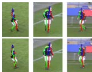
The method used by CVLAB means that a player's posture can be reliably represented in 3D using a single camera.
