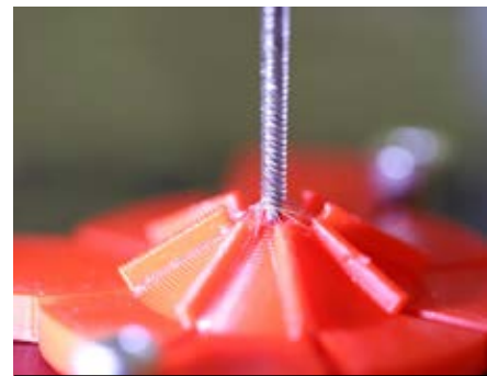
The pump structure is manufactured by winding copper and polyurethane wires around a steel rod, then fusing them together using heat.
