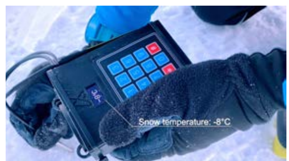
Device developed by students to correlate the skier's glide, ski preparation and snow conditions.
