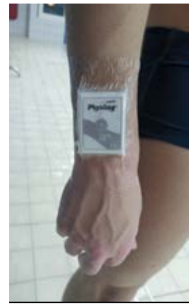
Body-fixed inertial measurement unit for the wrist.
