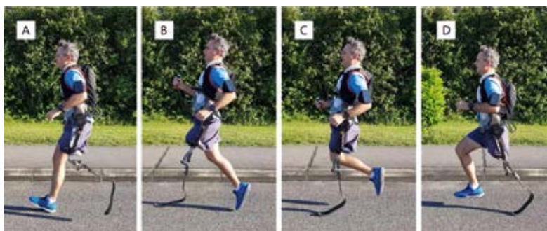
Running gait phases during testing with Sprint: (A) right heel strike, (B) flight phase, (C) left heel strike, and (D) left toe-off.
