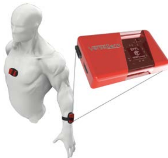
VersaSens is a multimodal biosignal monitoring wearable device (e.g., kinematic, ECG, PPG) that can be used during sports and daily activities.
