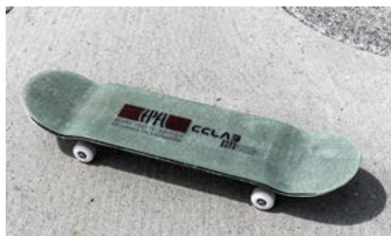
Skate made of FRP for modular rigidity and longer lifespan.
