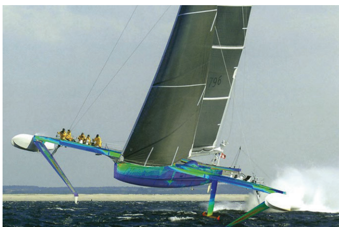
Stress and deformation simulation on the Hydroptère trimaran.
