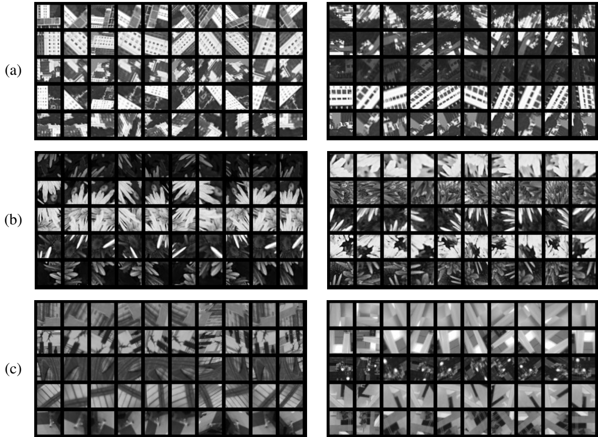
Fig. 6. Warped patches from the images of Figure 5 show the range of affine deformations we considered. In each line, the left most patch is the original one and the others are deformed versions of it. (a) Sample patches from the City image. (b) Sample patches from the Flowers image. (c) Sample patches from the Museum image.
