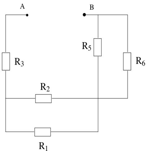
$$R_i = R_3 + \frac{R_1 R_2}{R_1 + R_2} + \frac{R_5 R_6}{R_5 + R_6} = \frac{85}{3} [\Omega]$$
