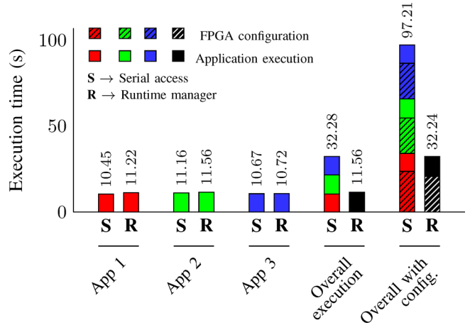
Fig. 3. Comparison between simultaneously sharing the FPGA with our runtime manager among multiple applications and serially providing exclusive use of the FPGA without PR.
