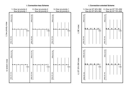
Fig. 5. End-to-End Delay for IDCT-ADD flow and MC-ADD flow in a connection-less and in a connection-oriented network
