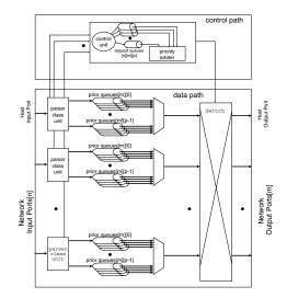
Fig. 3. Connection-less Priority-based Router.
