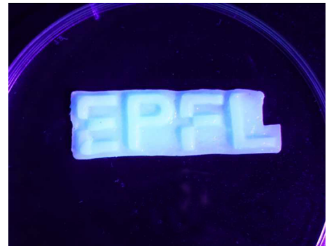
Figure 1. Photocured fluorescent biopolymer developed by ALCHEMY.
