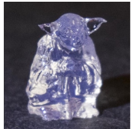
Figure 2. 3D structure printed in 30s with VAM at LAPD.
