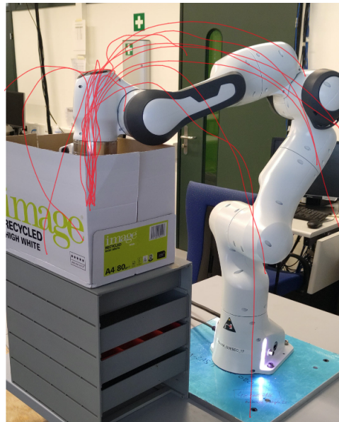
Figure 1: Experiment setup, with the panda robot at the attractor, and the demonstration dataset overlaid in red
