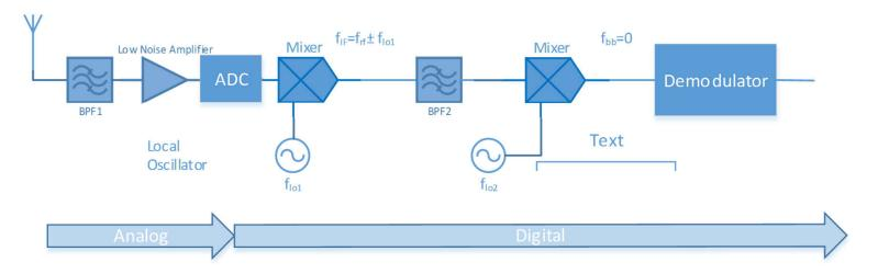
Advantage: the whole architecture of the digital part can be changed upon requirement, during operation, offering extreme flexibility.
