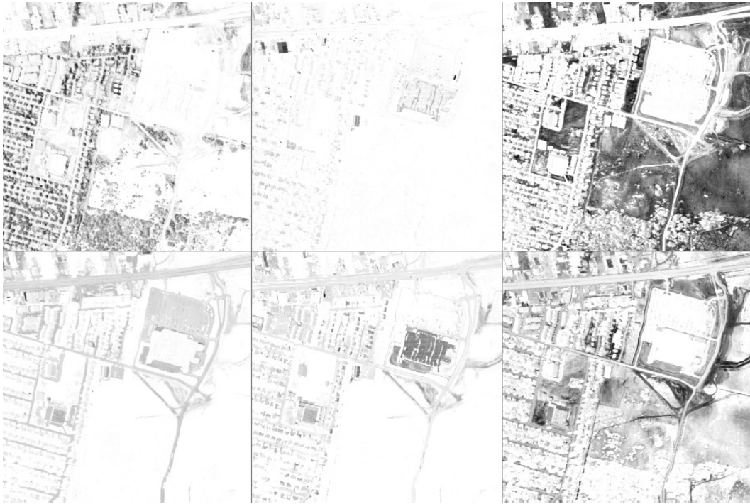
Figure 4: Abundance maps corresponding to the endmembers extracted by FGNSR-500 for the Urban HSI ( r = 6 ). From left to right, top to bottom: (i) trees, (ii) roof tops I, (iii) grass, (iv) road, (v) roof tops II, (vi) dirt.
