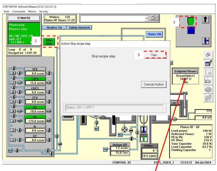
The system is fitted with integrated OES end-point system. Click on **"Endpoint Viewer" OceanOptics1** to open vision of the registered curve.
