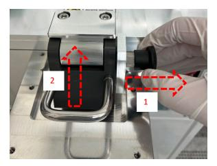
Load the wafer with its **main flat facing the rear of the loader**. Wafer rotation alignment is done visually.
