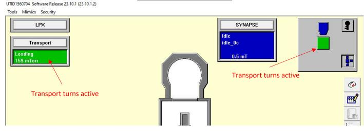
During the process, it is possible to stop the etch anytime when **Skip Step** is available: **1 Select Synapse module view**, click the **2 Skip Step** button, and **3 confirm the action.**
