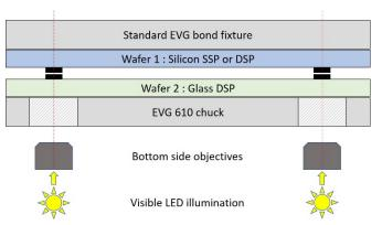
This configuration is used when one of the two wafers is transparent to visible illumination. It is the <u>default for anodic bonding</u> of borofloat and silicon wafers but can potentially be used with other types of bonding method.
