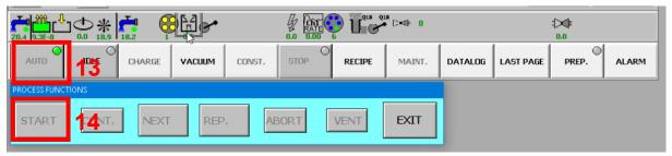
r) The pump-down is now starting. **Wait for the secondary pumping to start before leaving the tool.**
