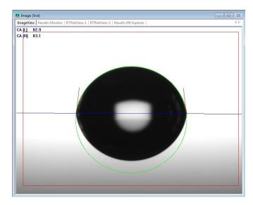
You can take several sets of measurements with different liquids. All measurements can be seen in the "Results Monitor" (main window). Please use the motorized Y-Axis ("Axes" tab) to move the wafer to a new position for a new dispense. Minimum distance between droplets should be 5mm.
