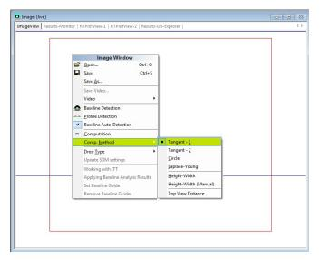
Take the measurement by clicking on "Computation" or "Run Computation Series". The series of measurements is set in the "Mode" tab of the control panel.
