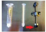
• Push the plunger into the disposable syringe. Rotate the holding clip to the top of the plunger. See image below.
