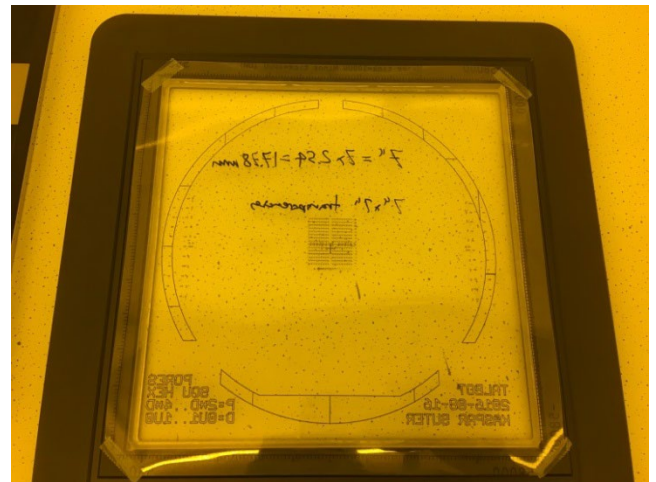
Figure 6: film attached with adhesives to glass plate
