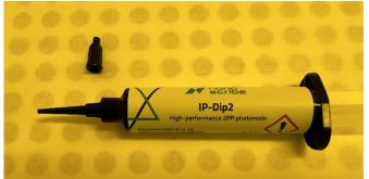
Dispense one drop at the sample center by gently pushing the cartridge piston. Spread out if necessary. After use, the tips should be cleaned after use by immerging in PGMEA for ~20 minutes and rinsing with IPA.
