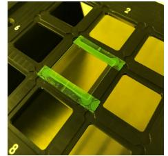
• Take your resist cartridge, remove the cap and screw in a dosing tip
