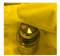
• <u>STEP 2:</u> Blow the lens with N2 gun to push the resist/oil from the lens. Wipe around the lens same as described above. Repeat several times.
