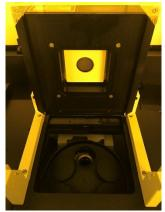
Objectives are inserted from the top. Remove the cap from the slot, insert the objective and rotate to screw it. Do not force and immediately inform the CMi staff if the objective is not rotating easily during the mounting.
