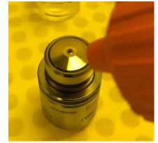
• <u>STEP 3:</u> Wrap one tissue around your index, hold the lens firmly and tilt it slightly as shown below.
