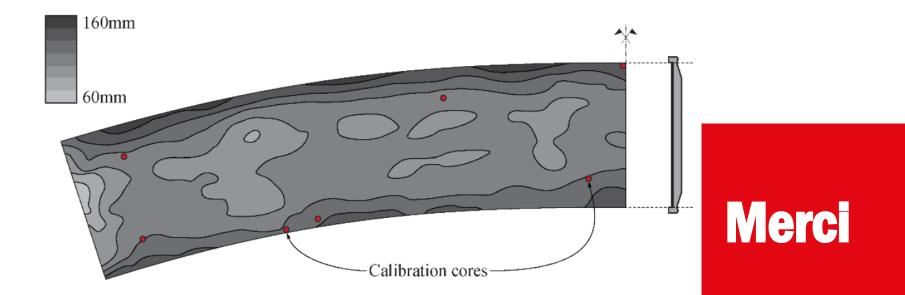
Typical thickness variability of pavement thickness on a slab bridge
