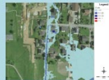
Fig. 4: Close up of the PC SWMM simulation for Courvaivre (La Combe) showing maximum water height (m).
