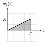
(a) Describe an ML receiver that decides which pulse was transmitted. The *n*-tuple former must contain a single causal matched filter. Finally, draw the matched filter impulse response.
