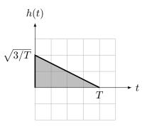
The output of the matched filter sampled at t = T and  $t = T + T_d$  is  $Y_1 = \langle R(t), \frac{w_1(t)}{\|w_1\|} \rangle$ and  $Y_2 = \langle R(t), \frac{w_2(t)}{\|w_2\|} \rangle$  respectively. The decision rule is
